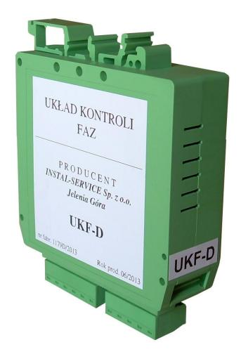
Relay of phase control type UKF-D 350 ... 550V, is designed to control the phase sequence and detect total decay of one or more phases in the three-phase supply grids of rated voltage of 350 to 550V.
